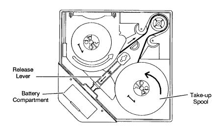
19. Slowly rotate the take-up spool counterclockwise three complete turns to secure the media onto the spool. Allow the release lever to return to its normal position.
