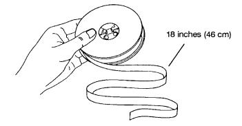
9. Lift the light guard and place the spool of media on the supply spindle with the number 1 side up.
